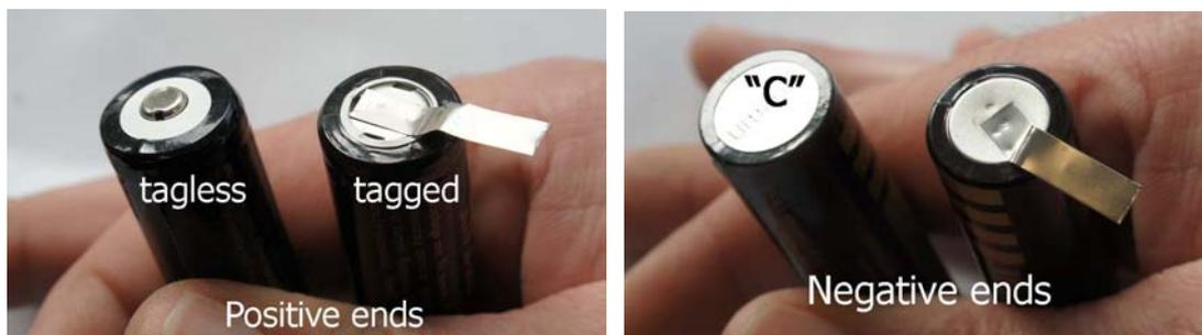
After removing the label from the tagless cell we can see a spot welded strip of metal going from the +ve to the -ve end on to a small thin circuit board. There is also some yellowish Sellotape to stop the strip touching the cell wall and causing a short circuit. Photo below right shows after cutting the strip to expose the PCB.
