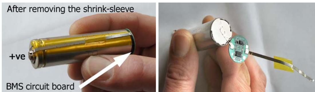
Clearly all we have to do to solder our own battery leads is to cut off the circuit board and throw it away, and shorten the spot-welded strips to form solder tags, or alternatively to leave the PCB in place and solder to the free tag.
