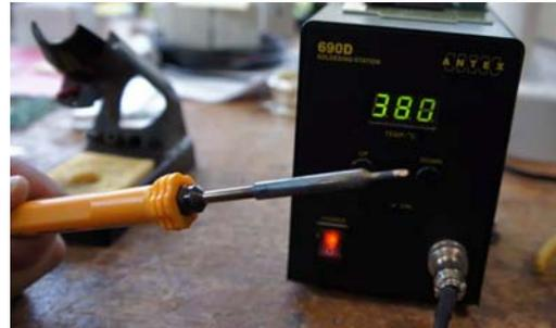
Then the battery cap needs to be fluxed and tinned with solder. One drop of the Warton flux is being applied using the end of the file and allowed to dry. Lead solder is at the ready and it takes only a couple of seconds to coat the battery cap all over with solder. Strip the wire you want to solder to the cap, twist the inner fibres on each other, and tin that, and finally trim the metal end of the wire to 3mm.
