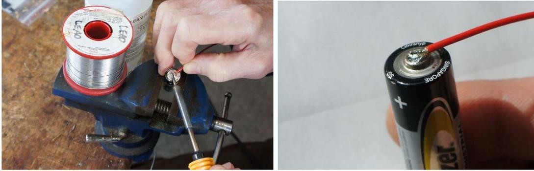
Clean the tip of your soldering iron with a damp sponge to remove all old solder blobs and then tin it with a tiny amount of fresh solder. Put the tinned wire in contact with the tinned cap. Quickly dab them with the tinned soldering iron for only a couple of seconds and the solder will flow together across the joint leaving a very tidy and strong joint in a process which has not subjected the battery itself to significant heating.
